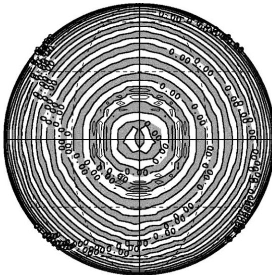
Fig. 6. Height error after one rotation for Test Case 1 with \alpha = \pi/2 - 0.05 . The contour interval is 1.25 m. Negative regions are shaded.
